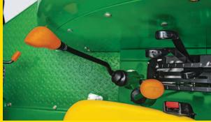
Transmission is offered with either 9 forward and 3 reverse speeds or 12 forward and 12 reverse speeds with PowrReverser for fast headland
