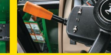
PowrReverser transmission has wet clutch to ensure maximum durability and long life. PowrReverser enables the operator to reverse without clutch, the result is less pedal clutch operation per day.
