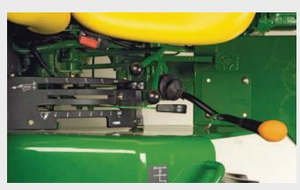
Transmission with 9 forward and 3 reverse speeds to perform fast headland turns thanks to inline shifting: The second gear is positioned directly on the opposite side of the reverse gear, so that the operator can use inline shifting like a reverser.
