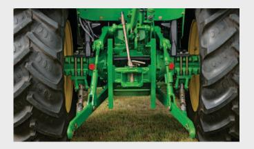
Inboard planetary final drives distribute rear axle loads over three points for reduced stress on individual gears and shafts: for a longer tractor life, less service and more uptime. Max. lift capacity of 1,800 kg (at balls).
