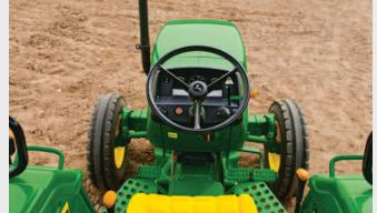
For enhanced visibility, the exhaust muffler has been placed inside the hood to give you a clear and unobstructed view from the driver's seat.
