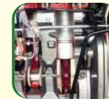
Oil Jet for Piston Cooling
